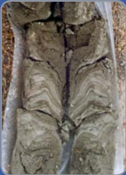
■ Mine tailing core sample
