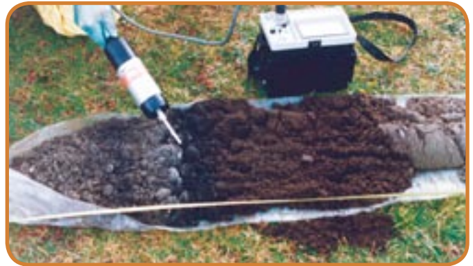
■ Field testing with a gas detector
